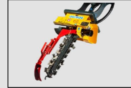
Available with bucket, bit tool or mixed digging chains
